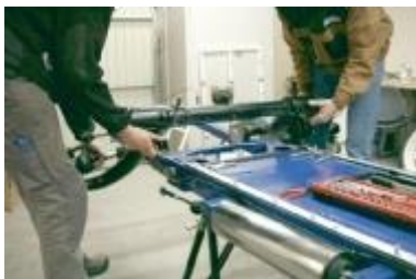
Mounting the axle tube
