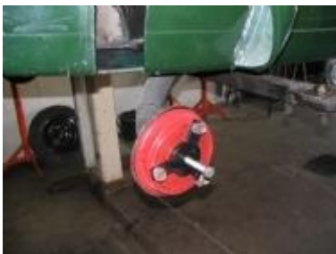
Pulling the brake drum
