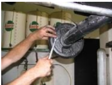
Back off brake adjuster cam
