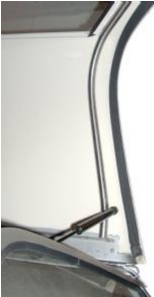
Mossrubber on edge windowframe/door
