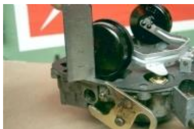
Float level adjustment
