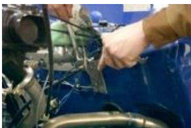
Clutchcable adjustment
