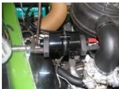
Ignition coil on bracket
