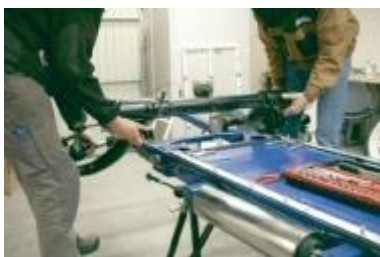
Mounting the axle tube
