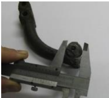
Steering arm ball joint
