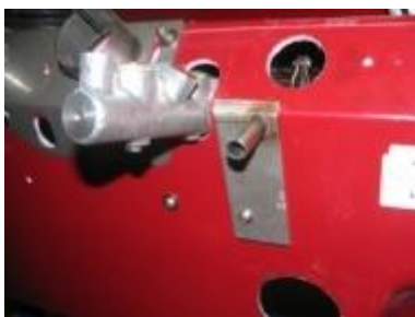
Clutchcable connection
