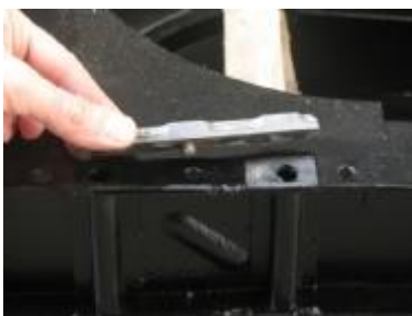
Spacer rear suspension
