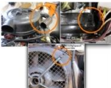
1: Pipe on the airbox, mounting point behind the Fan-cover, remove the throttle-spring and -clip.
