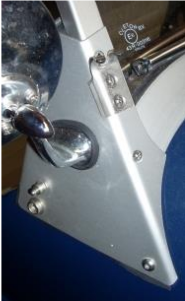
fig. 2 Attach hook to windscreen
