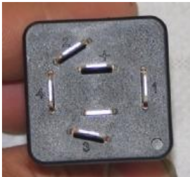
Connections light switch
