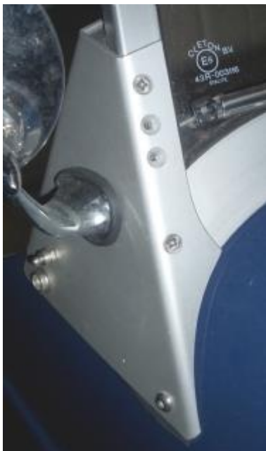
fig. 1 Undo 2 screws from windscreenframe
