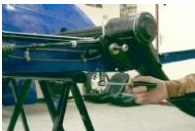
Mounting axle tube
