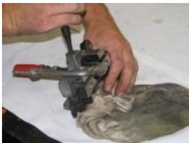
Pressing the piston out using compressed air
