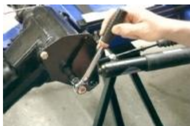
Shockabsorber mounting
