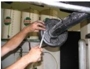
Back off brake adjuster cam
