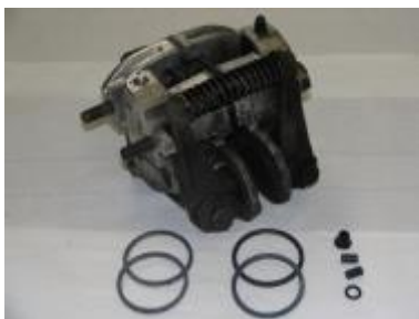
Old calliper with overhaul set
