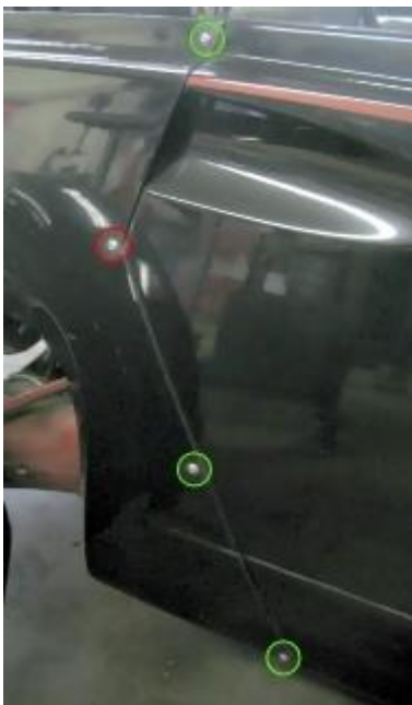
Bolting the front to the body
